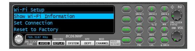
7. You will now see 4 items listed on the BCD536HP LCD window. The second item is the IP address that has been assigned to the BCD536HP by your home router. Write this number down as it will be needed later when setting up the Wi-Fi stream (feed) in ProScan.
